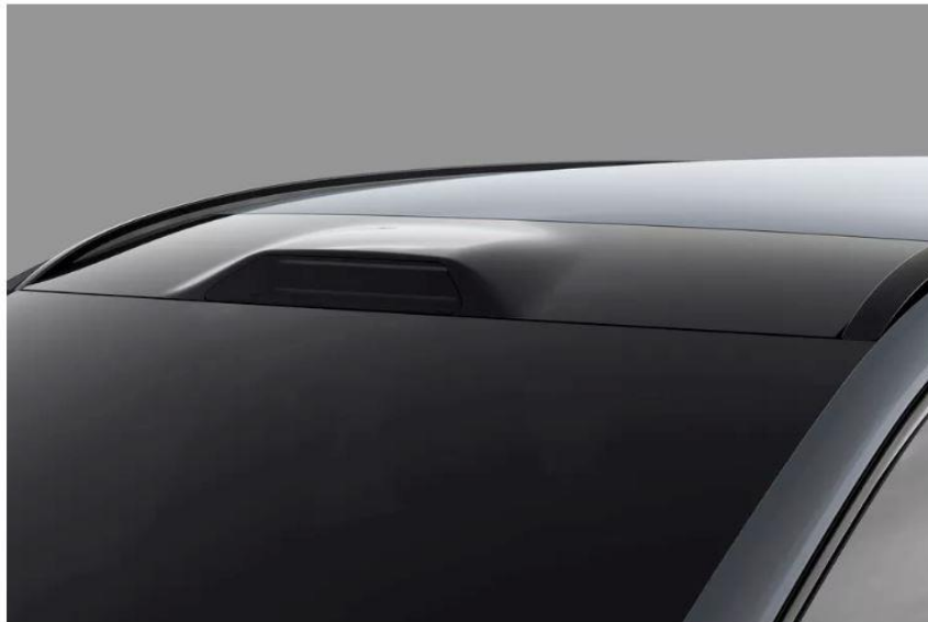
Volvo says Luminar's LiDAR will be "seamlessly integrated" into its vehicles. | Photo: Volvo
